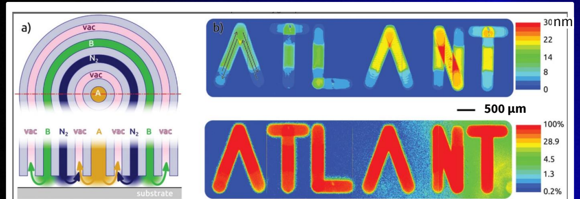
Illustration of \mu DALP™ nozzle geometry and process principles (left), ellipsometry thickness map and low-energy ion scattering spectroscopy map of Pt deposition Ref: Small Methods 2022 , 6, 2101546
